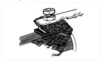
**8.8** Wrap two layers of 2" (51 mm) #50 tape over shield connectors and studs.
