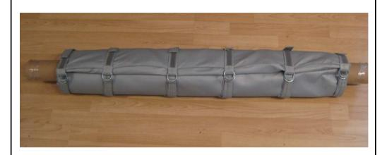
3M STFF 14W – hsb sleeve shield with shirt cuff carrier & laminated, heat shield barrier 12mm standard cable sleeve in centre of the specimen 3M protect mat 1100mm long, 820mm wide.
